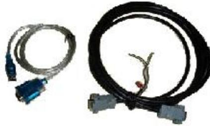
fig 5 USB-RS232 Cable and Serial Cable
